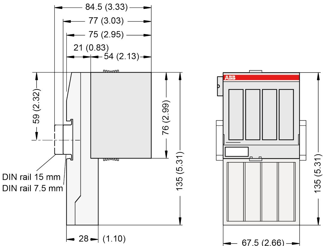
*The dimensions are in mm and in brackets in inch.*
